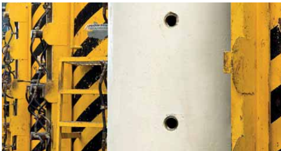
Rigid, mould-injected PU insulating material
