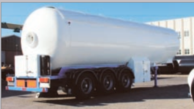
47 m 3 LPG tanker with transfer equipment
