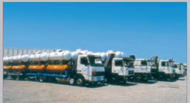
LAPESA crane trucks for deliveries of LPG tanks
